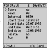
The activated recording is shown at the right of the top line.
